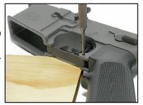
If it was removed earlier, insert the safety detent into the receiver. Insert the safety detent spring into the SE-1. Place the SE-1 onto the grip tang, aligning the safety detent spring with the corresponding receiver hole. Carefully compress the spring as you fully seat the SE-1 onto the receiver, making sure the spring does not bend.
