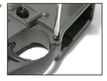
Slide the old grip off while carefully removing the safety detent spring. If possible, leave the safety detent in the receiver, but be aware that the detent will fall out if the receiver is held upright.
