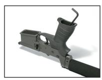
THE SAFETY DETENT SPRING AND SAFETY DETENT ARE RETAINED BY THE GRIP AND WILL BECOME LOOSE WHEN THE GRIP IS REMOVED. Using an appropriate screwdriver or wrench, remove the grip screw. Do not re-use the old grip screw or washer with the SE-1, use supplied hardware only.
