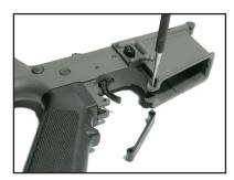
Slide the lock washer onto the grip screw. Put the grip screw on the end of a long 3/16 inch hex wrench and insert the screw into the hole at the top of the grip cavity. Carefully thread the screw into the receiver. Using excessive force may damage the receiver threads. If the screw binds, stop, back it out and try again.
