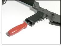
Using a small flat blade screwdriver, install the supplied trigger guard screw into the front of the trigger guard.
