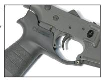
Using the punch, depress the spring pin on the front of the trigger guard and then disengage the trigger guard from the receiver.
